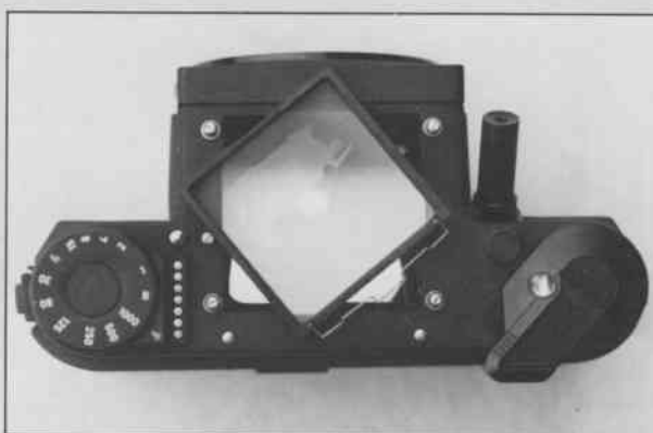
Above left: The meter prism is a shutter-priority system with a light-balancing LCD display. Triangular marks indicate the aperture range.
